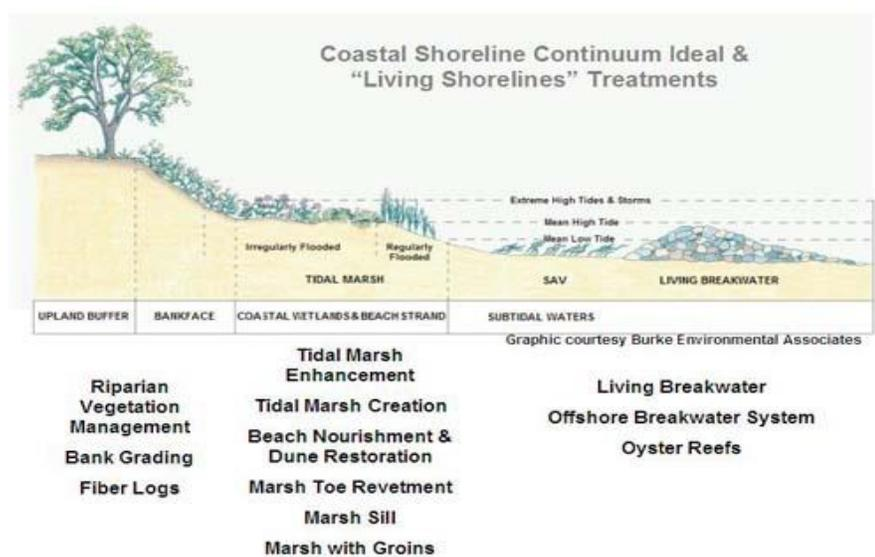
Shorelines are often stabilized with hardened structures, such as bulkheads, revetment, and concrete seawalls. Ironically, these structures often increase the rate of coastal erosion, remove the ability of the shoreline to carry out natural processes, and provide little habitat for estuarine species. Living shorelines use plants, sand, and limited use of rock to provide shoreline protection and maintain valuable habitat.
